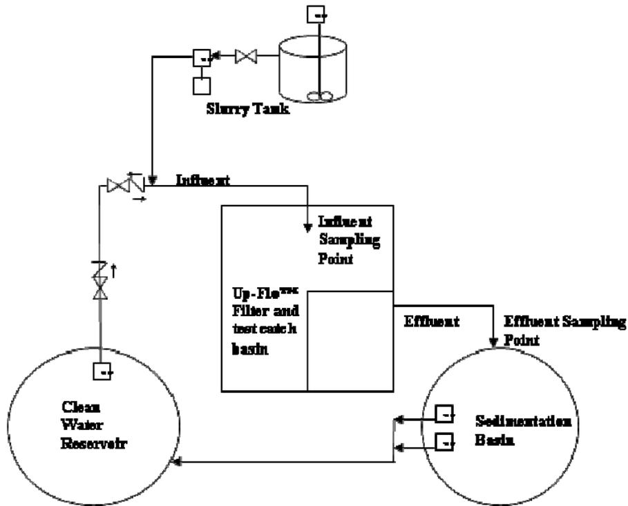
Up-Flo® Filter System as tested in the Laboratory
