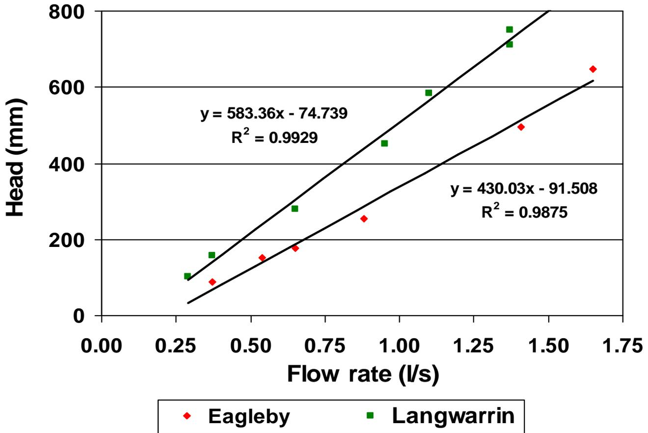
Figure 2 – Head discharge characteristics for filter sands sourced from Rocla Pty Ltd
