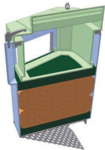
**Figure 5:** Cut-away view of the Filter Module
