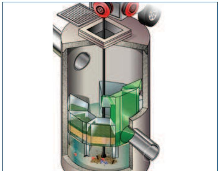
**Figure 4:** Sediment is removed with a vactor hose
