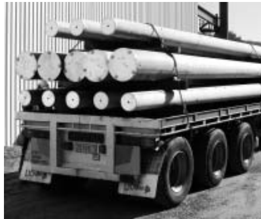
Poles with same tip diameter are placed together butt-to-butt
