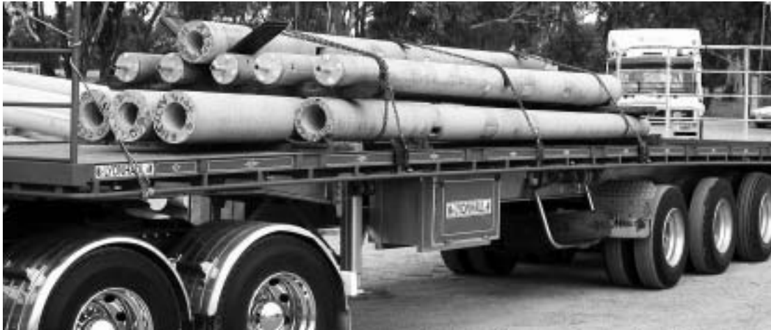
Longer poles should be placed on bottom layer
