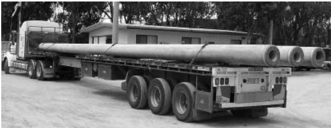
Use extendable trailer for poles or piles longer than 14m
