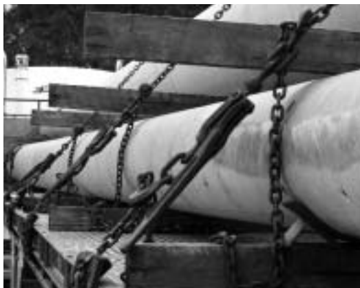
Align fastening with timber bearers
