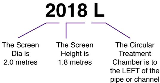
Check that the CDS® Unit model supplied is that which is specified on the project drawing and that the relevant Rocla Water Quality Operation and Maintenance manual has been provided.
