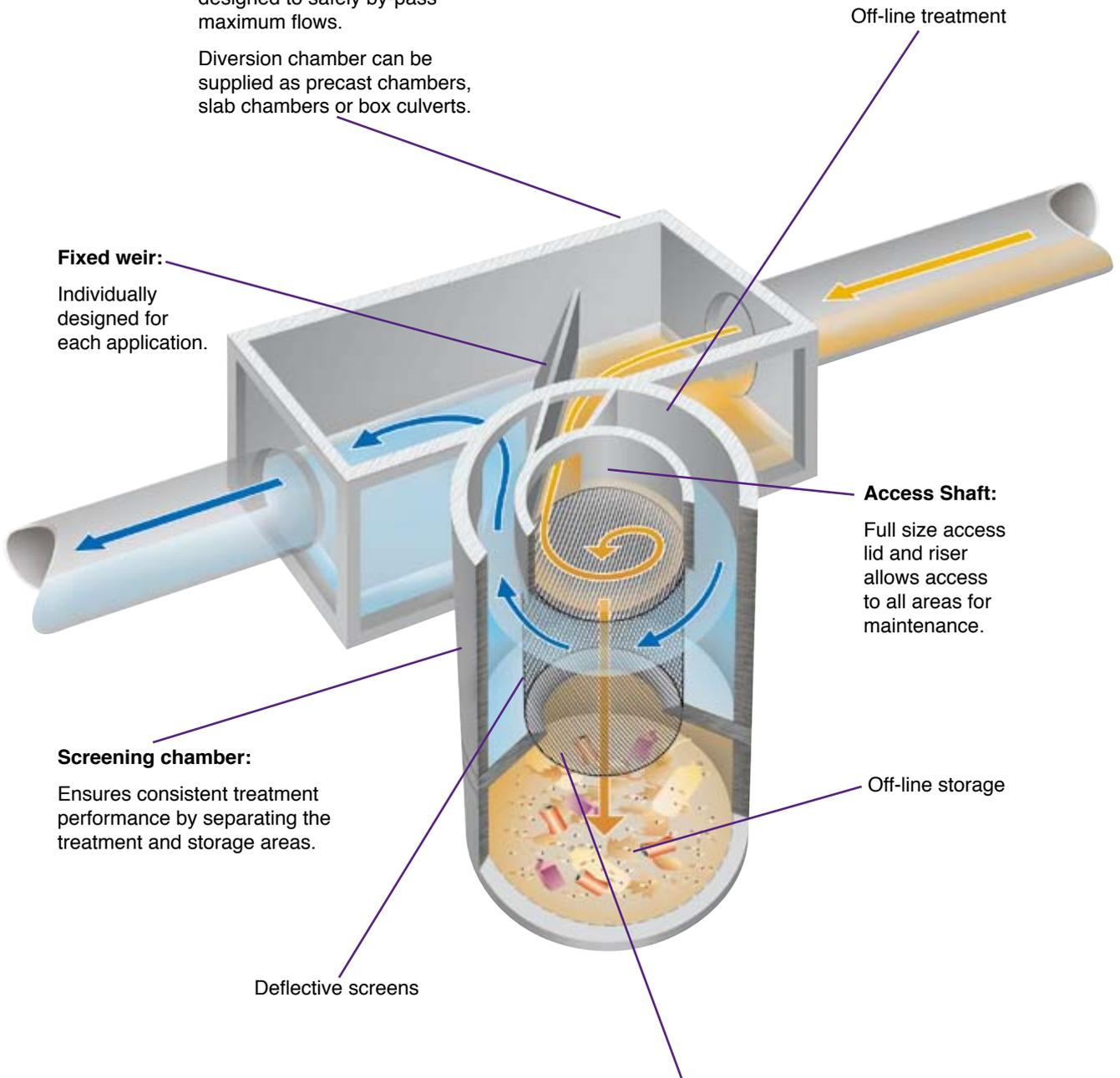
Figure 2: Key features of CDS® Units
