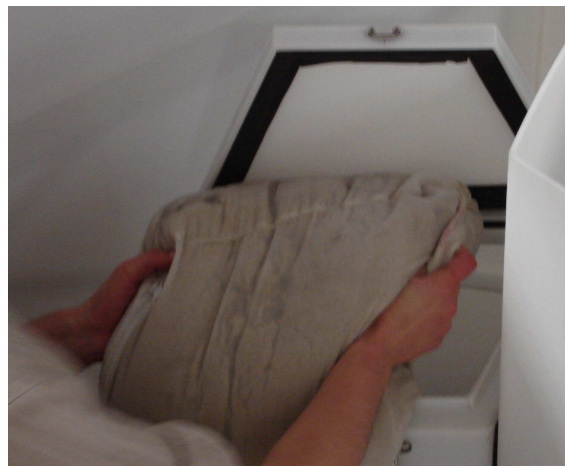
Figure A-5: View showing media bag with Filter Sand being installed in the Filter Module
